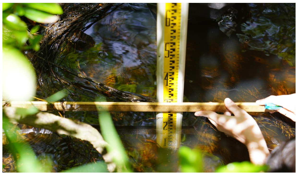
Figure 2: The horizontal distance between the vertical surveying rod and the face of the bank being measured using a ruler and line level.
